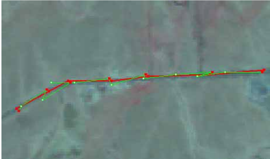
Figure 1: Random spikes produced in areas where roads are not easily detectable (much of East Africa) and when using default parameter settings
